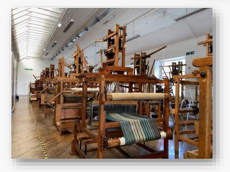
6 - A more traditional loom, which has the advantage of having parts that can be manufactured to replace. The noise of many of these looms operating in one open space can be problematic, and noiseprotection is advised.
