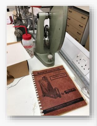
1 - A stelometer, which measures strengthelongation characteristics. The machine appears to date to the 1950s or 60s.
